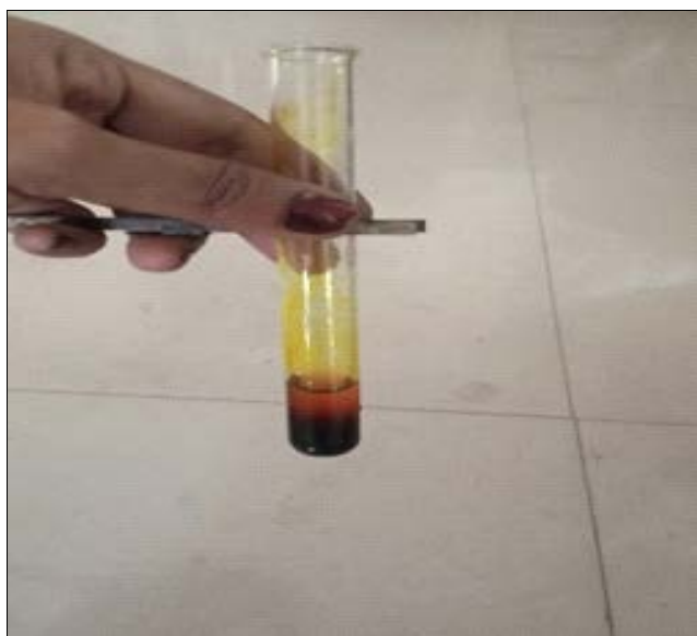
Fig 12: Tannins test for Coconut oil
